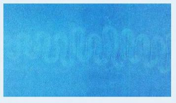
manner as to aim the plastic straight into an open area. The plastic launches out into the open mold cavity like a piece of "silly string" and then stacks up in squiggles.
