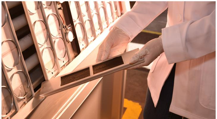
QUV testing allows for the development of high performance coatings.
